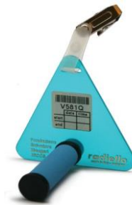
Figure 23: Typical setup of passive diffusive samplers
